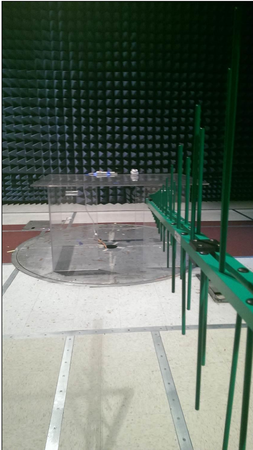
Photograph 4. Radiated Emission, Test Setup
