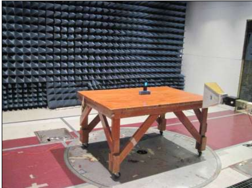
Photograph 8. Radiated Spurious Emissions, 1 GHz – 18 GHz
