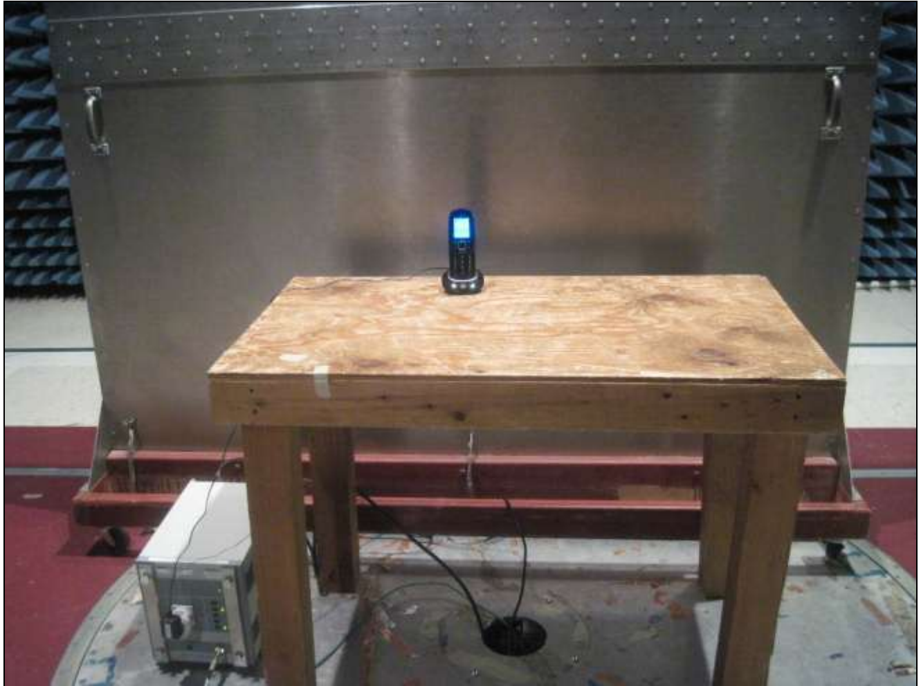
Photograph 6. Conducted Emissions, 15.207(a), Test Setup
