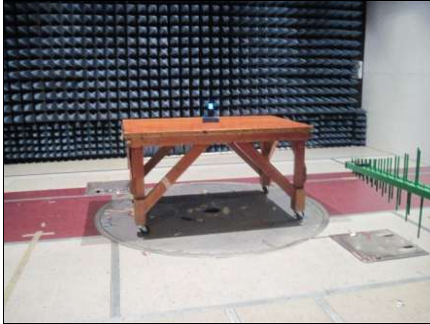
Photograph 7. Radiated Spurious Emissions, 30 MHz – 1 GHz
