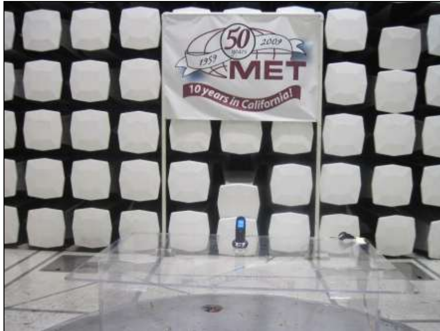
Photograph 5. Radiated Emissions, Test Setup
