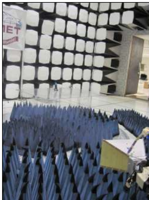
Photograph 4. Radiated Emissions, Test Setup, 1 GHz – 18 GHz
