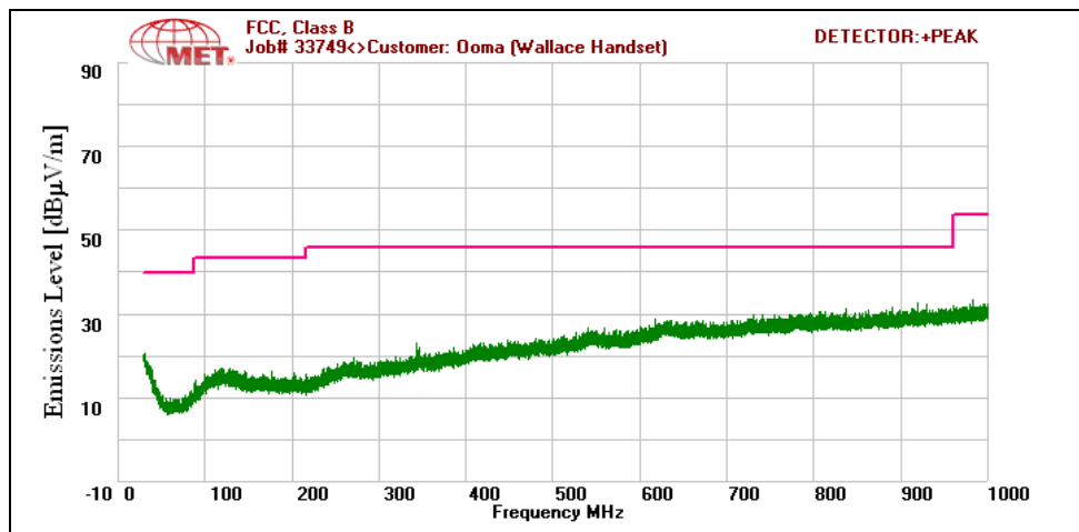
Plot 14. Radiated Spurious Emissions, Mid Channel, 30 MHz – 1 GHz
