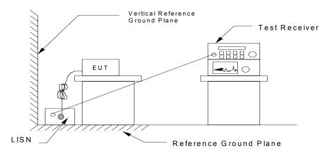
Test Set-Up 4
