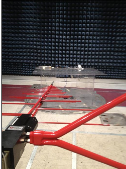
Photograph 7. Radiated Emission, Test Setup, Ooma Telo, 30 MHz – 1 GHz
