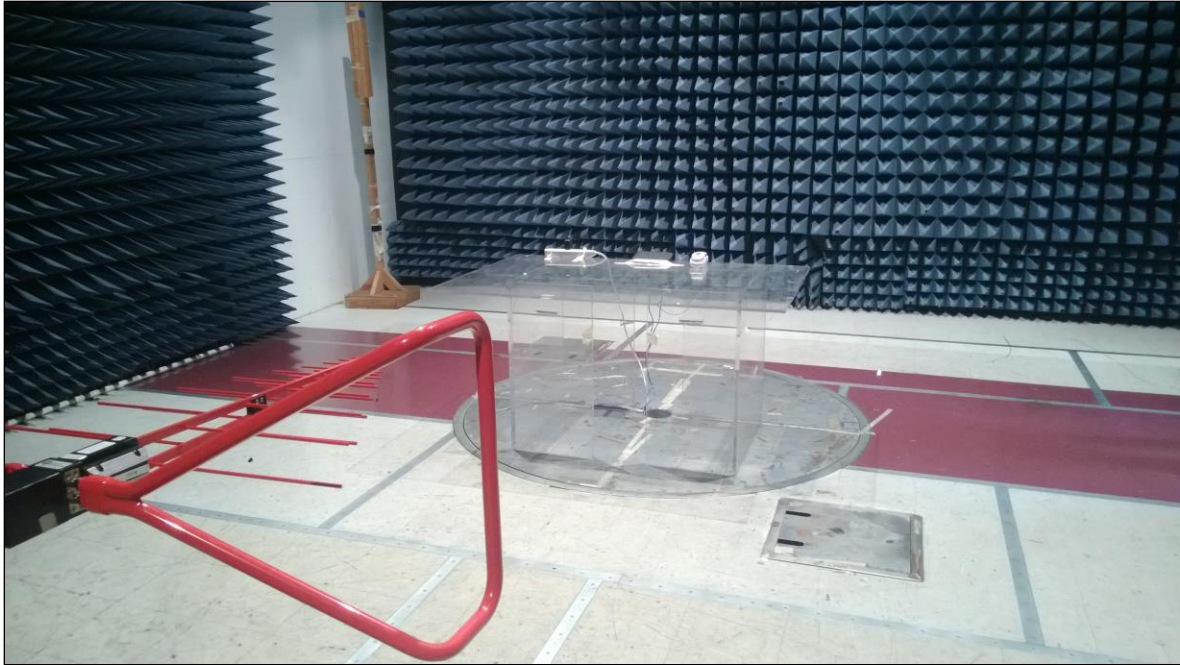
Photograph 9. Radiated Emission, Test Setup, Ooma Telo 2, 30 MHz – 1 GHz
