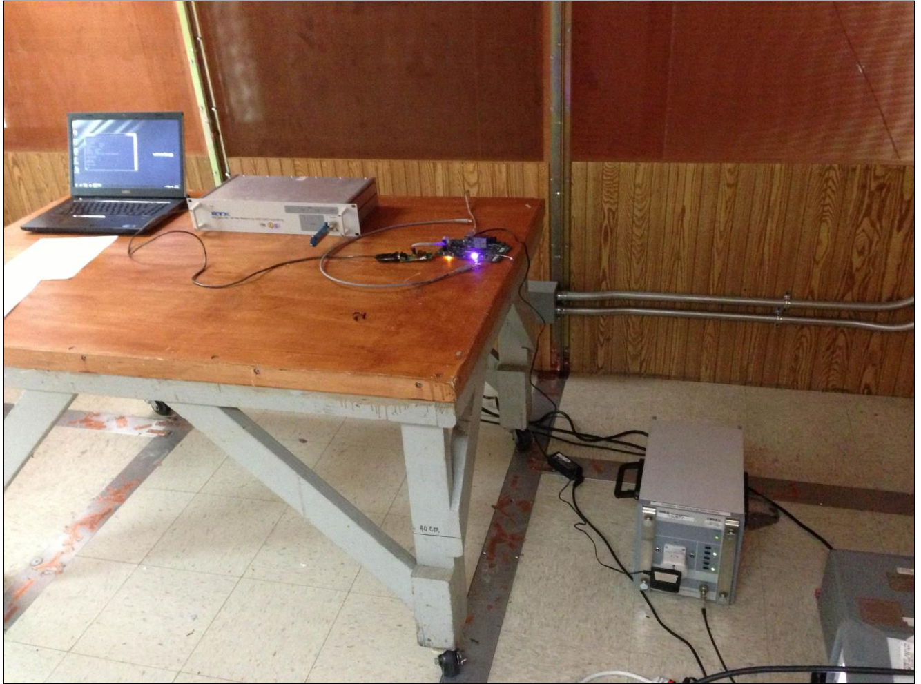
Photograph 11. Conducted Emissions, §15.315, Test Setup
