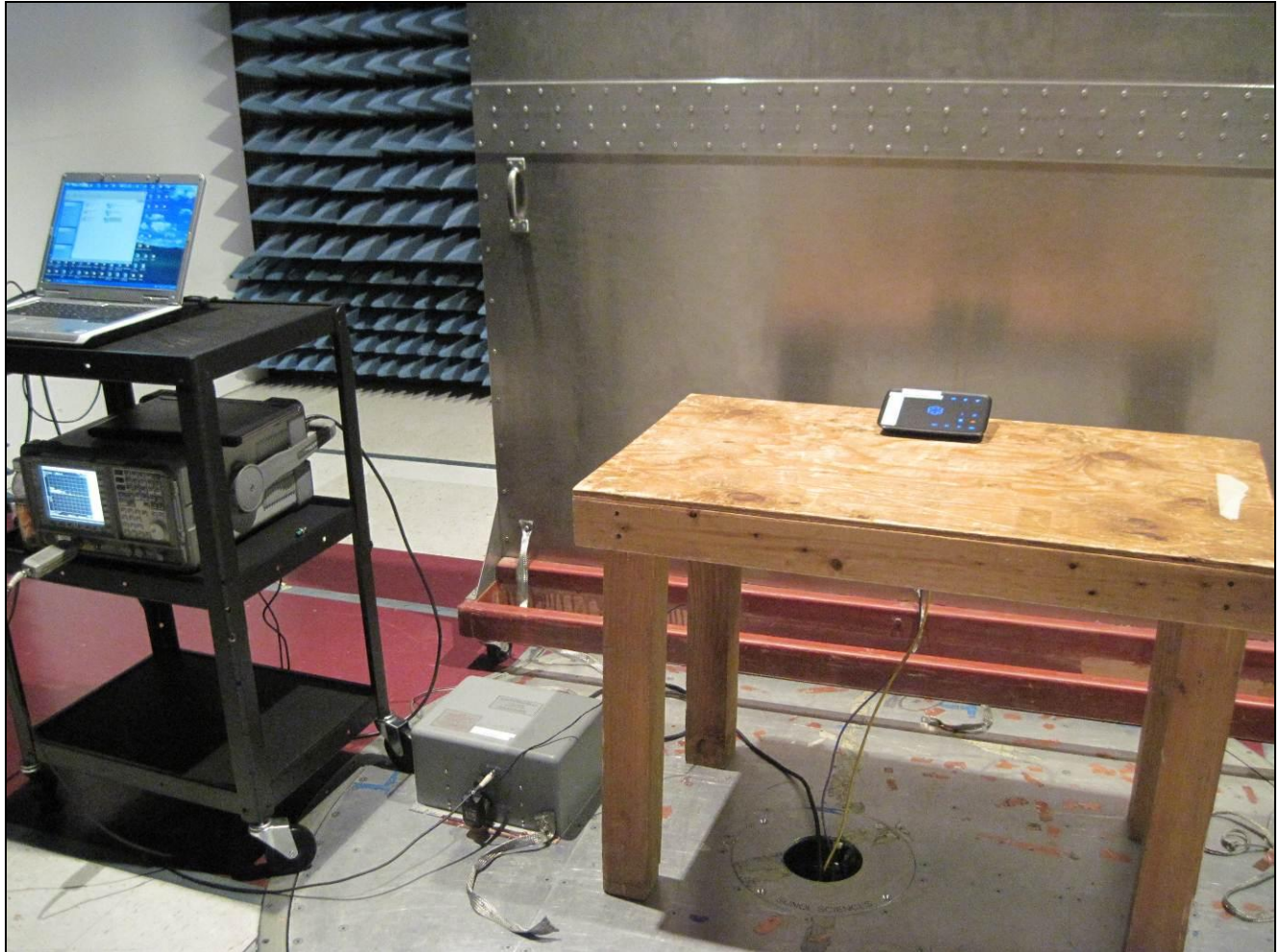
Photograph 5. Conducted Emissions, 15.207, Test Setup
