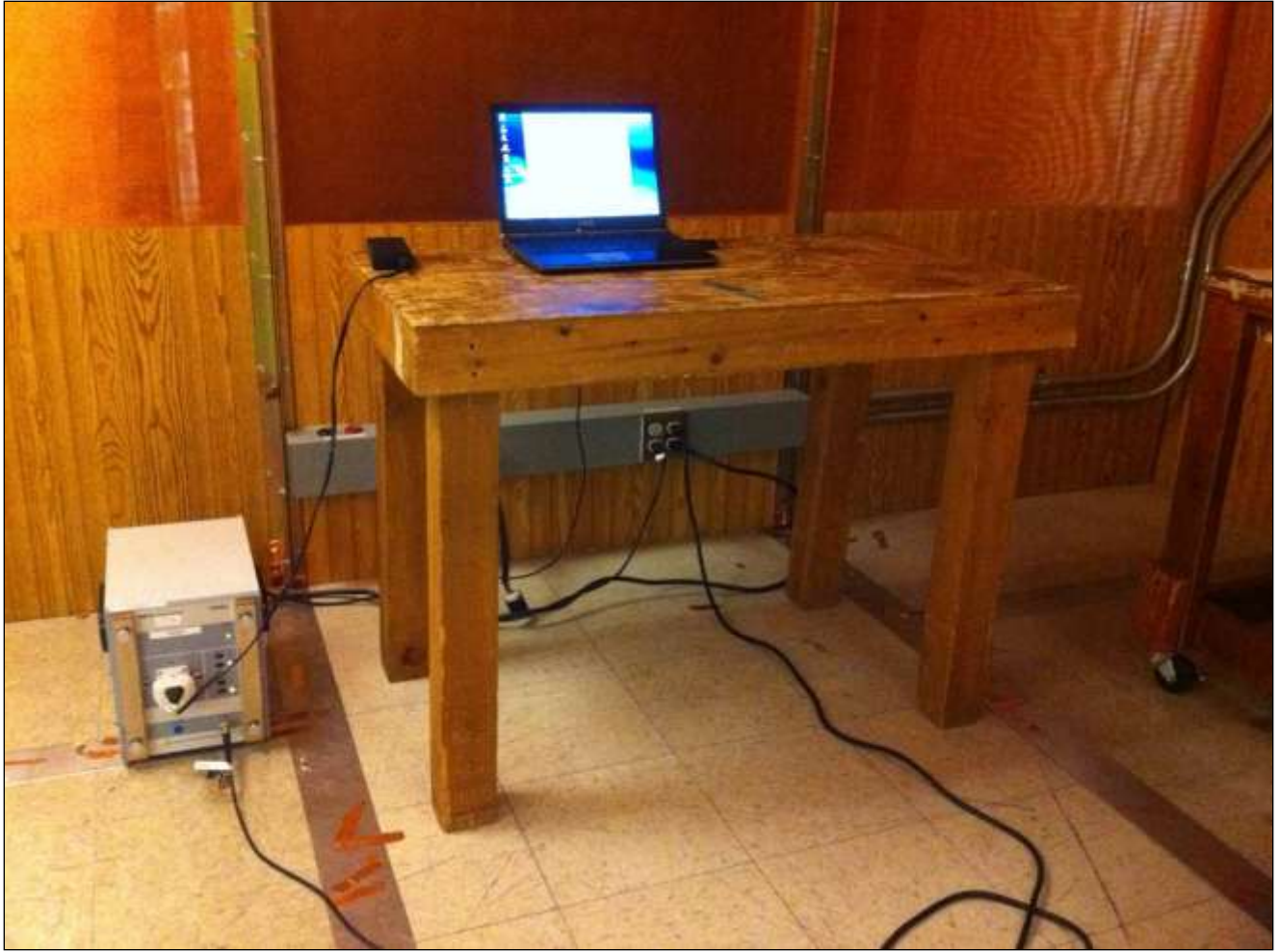
Photograph 6. Conducted Emissions, 15.207(a), Test Setup
