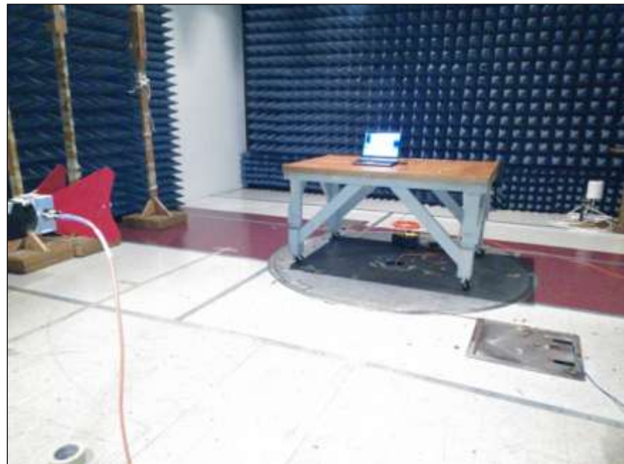
Photograph 8. Radiated Spurious Emissions, Test Setup, 1 GHz – 18 GHz
