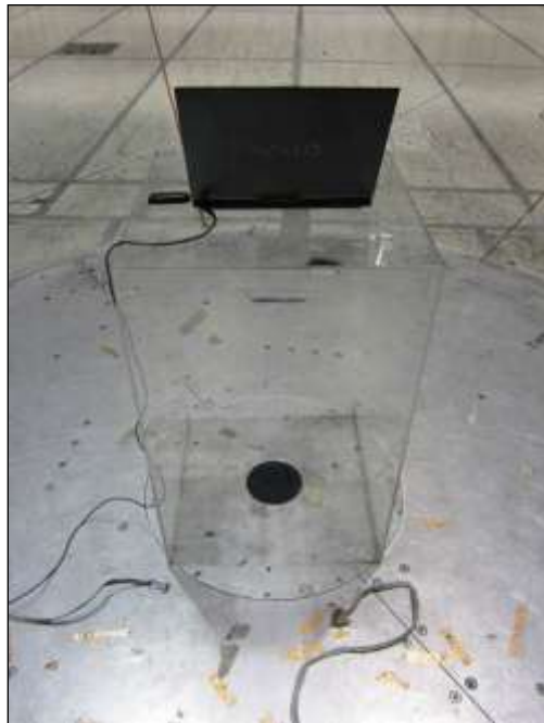
Photograph 5. Radiated Emissions, Test Setup, Rear View
