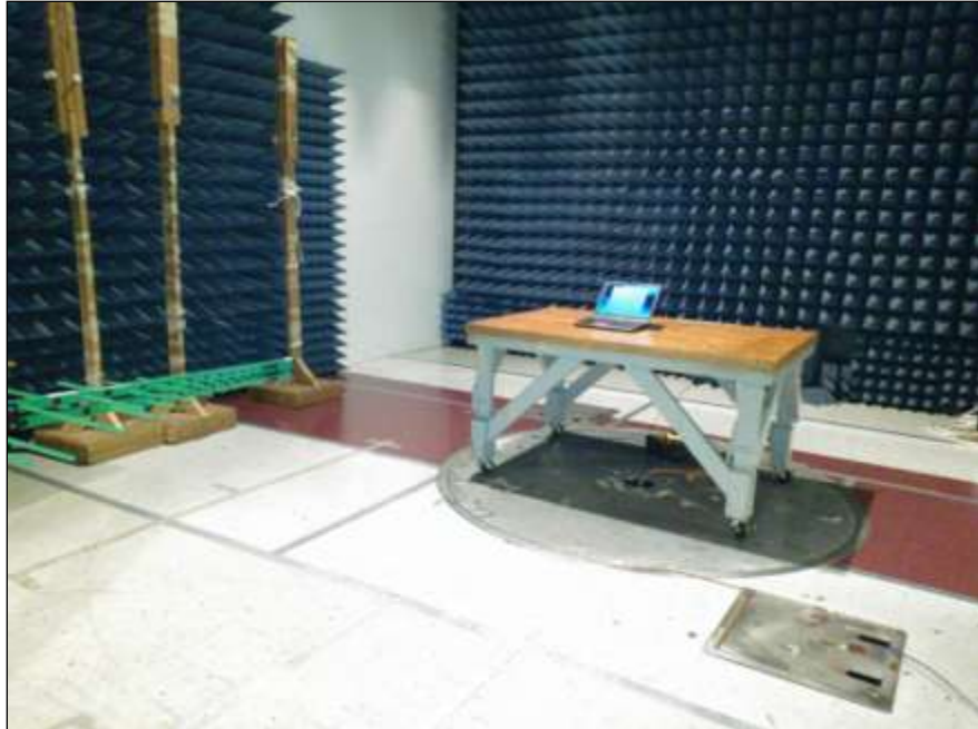
Photograph 7. Radiated Spurious Emissions, Test Setup, 30 MHz – 1 GHz
