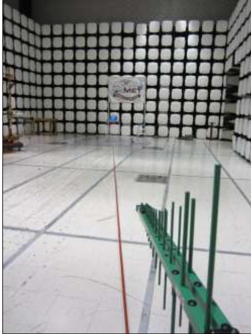
Photograph 2. Radiated Emissions, Test Setup, 30 MHz – 1 GHz
