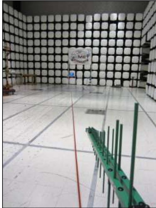
Photograph 3. Radiated Emissions, Test Setup, 30 MHz – 1 GHz
