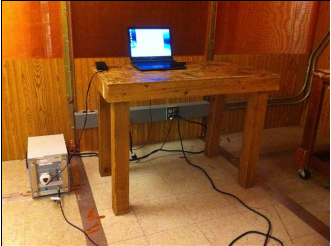
Photograph 7. Conducted Emissions, 15.207(a), Test Setup
