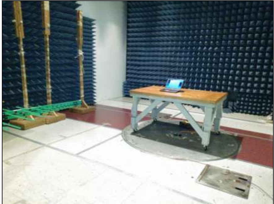
Photograph 8. Radiated Spurious Emissions, Test Setup, 30 MHz – 1 GHz
