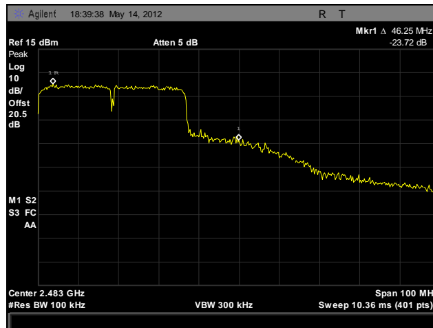
Plot 130. Conducted Band Edge, High Channel, 802.11n 40 MHz
