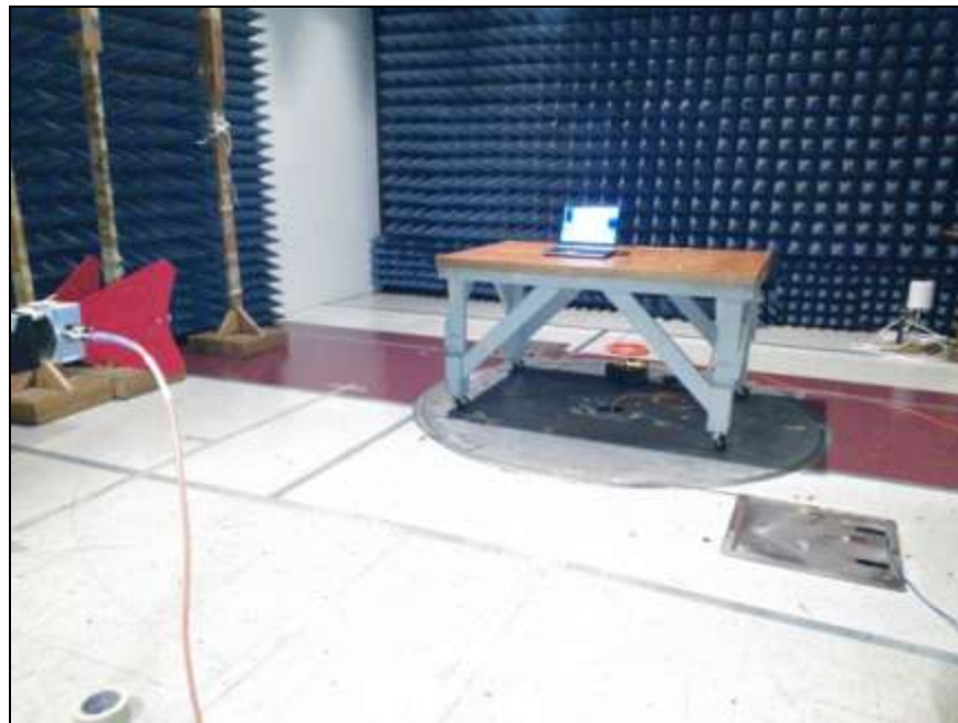
Photograph 11. Radiated Spurious Emissions, Test Setup, 1 GHz – 18 GHz
