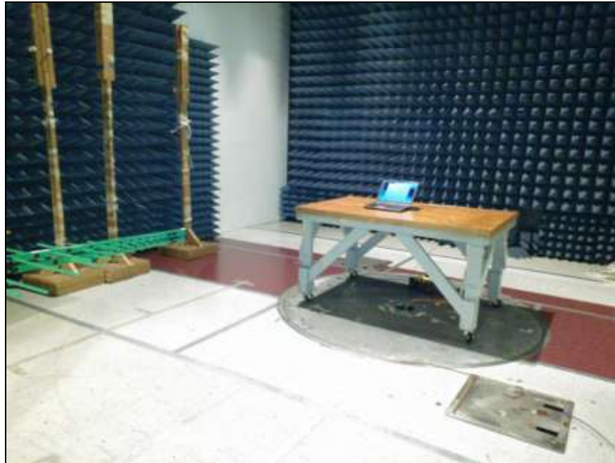
Photograph 10. Radiated Spurious Emissions, Test Setup, 30 MHz – 1 GHz
