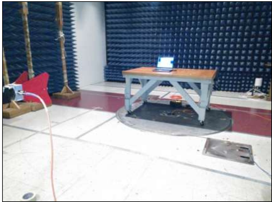
Photograph 9. Radiated Spurious Emissions, Test Setup, 1 GHz – 18 GHz
