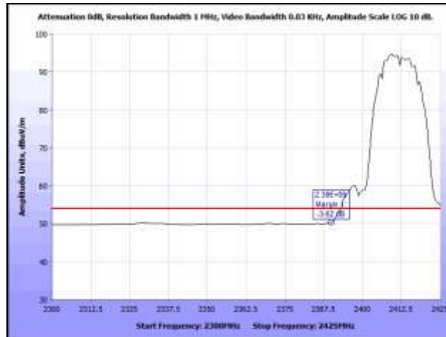
Plot 83. Radiated Band Edge, 802.11b, Low Channel, Average
