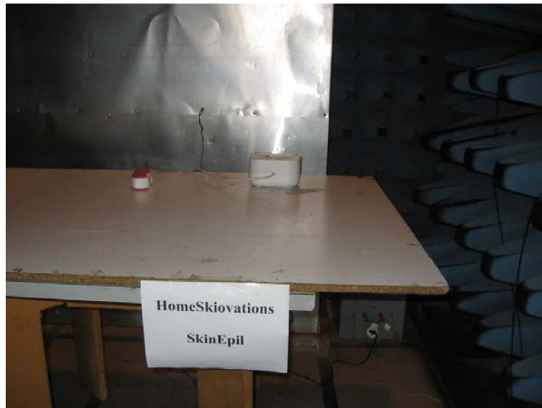
Figure 2. Conducted Emission Test
