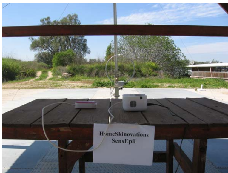
Figure 3. Radiated Emission Test
