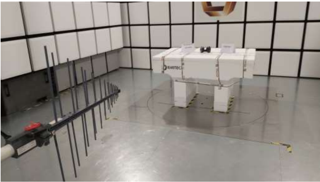
TEST SETUP PHOTO(S) – TX MODE – 200MHZ TO 1GHZ
