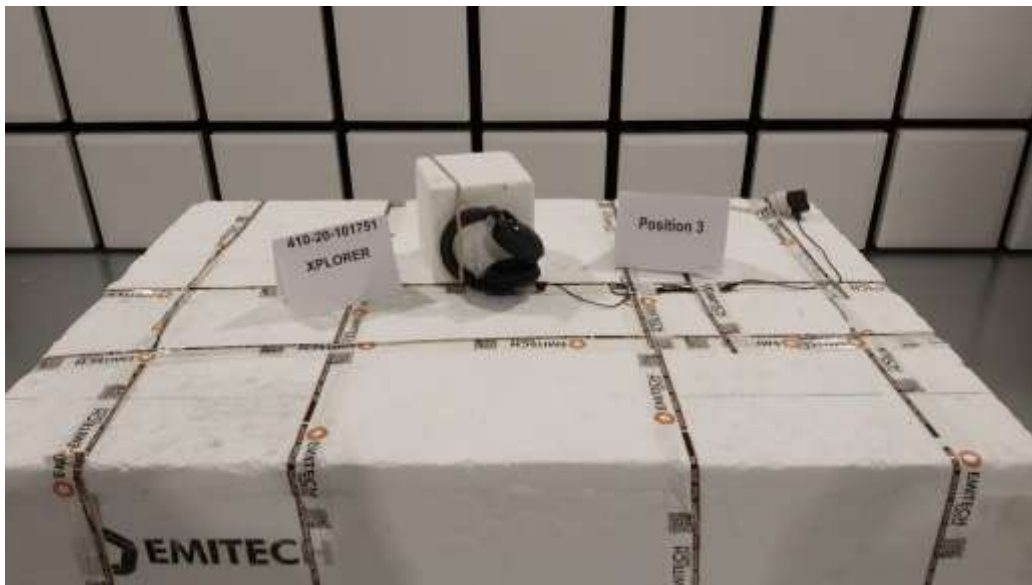
TEST SETUP PHOTO(S) - CHARGING + RX MODE – POSITION 3
