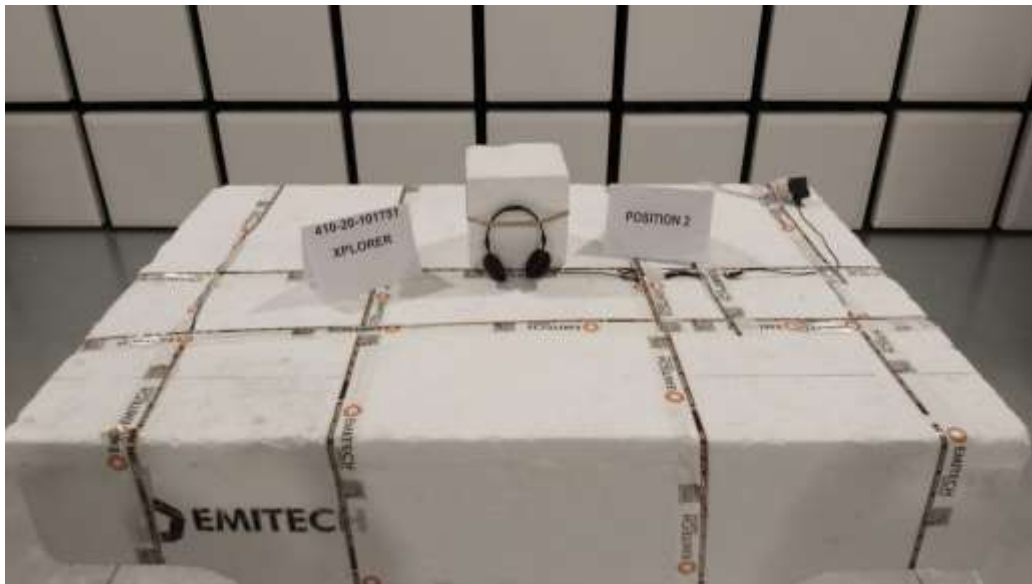
TEST SETUP PHOTO(S) - CHARGING + RX MODE – POSITION 2
