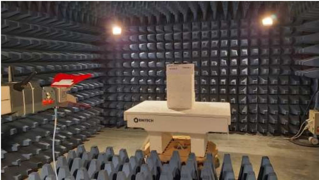
TEST SETUP PHOTO(S) - EIRP
