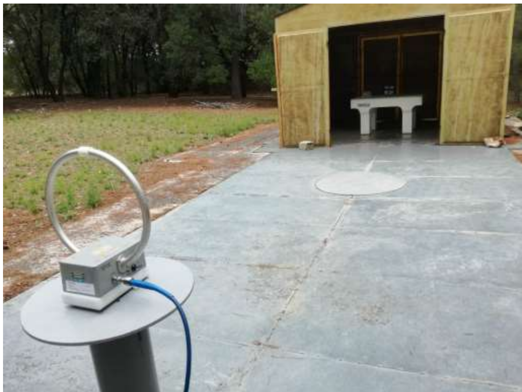
TEST SETUP PHOTO(S) - (OATS) - FOR FREQ 4.1KHZ
