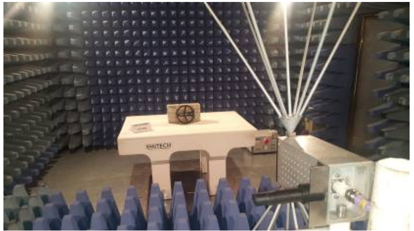
Radiated pre measurement
