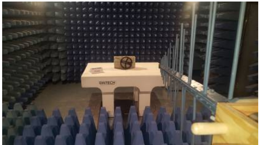
Radiated pre measurement
