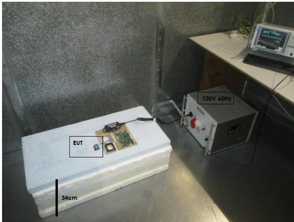
AC Power Line Conducted Emissions, Test set up
