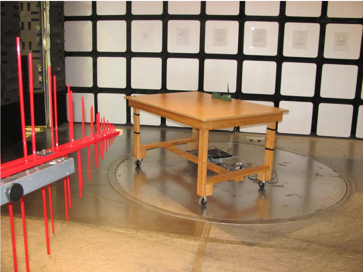
Illustration 1: Radiated emission setup – photo 1
