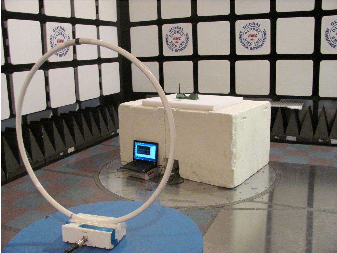
Illustration 2: Radiated emission setup - photo 2
