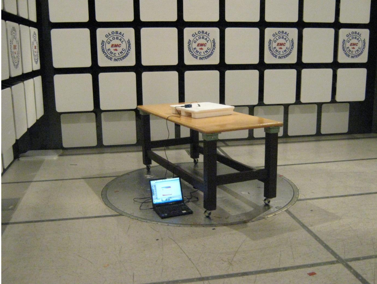
Figure 1 – EUT Radiated emission setup
