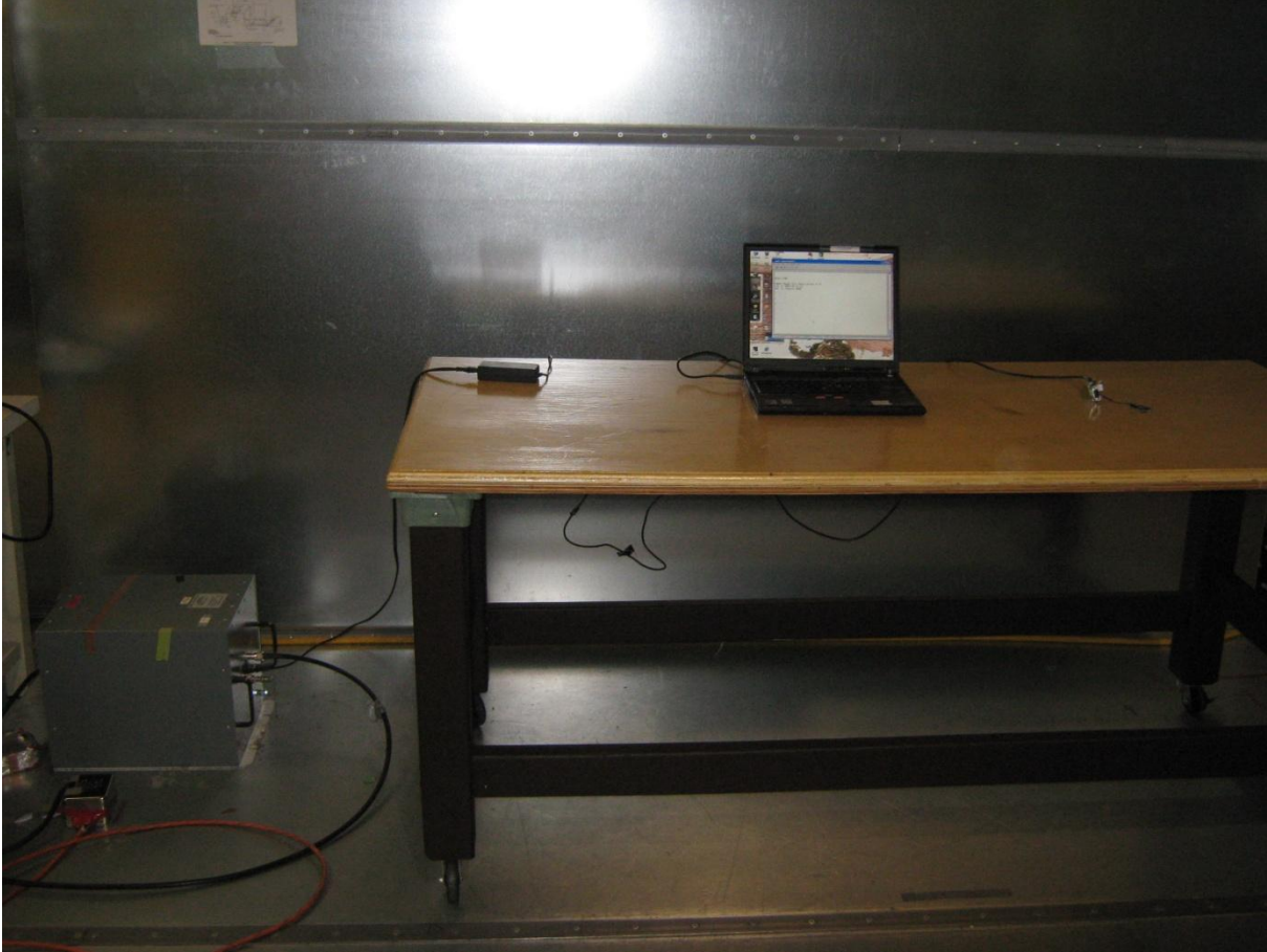
Figure 2 – Conducted emission setup
