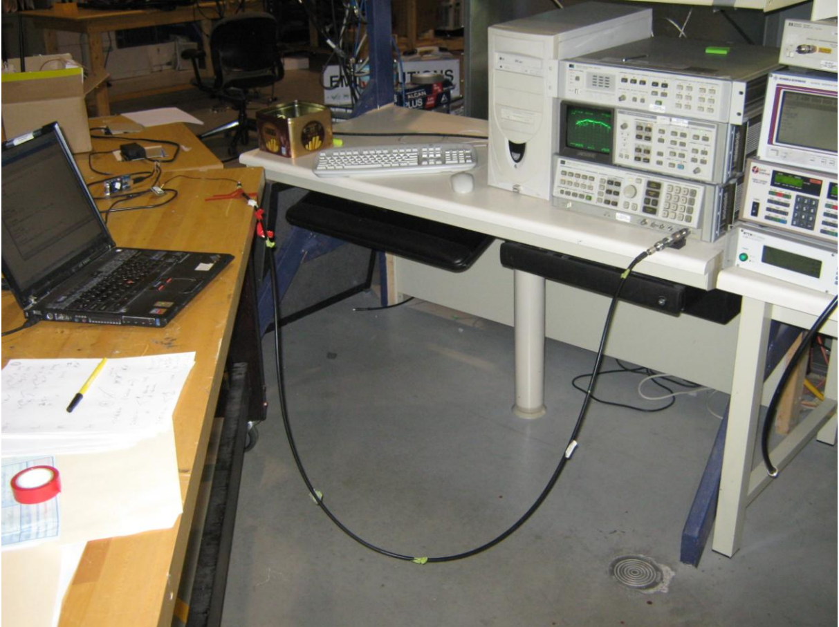
Figure 4 – Conducted power emissions
