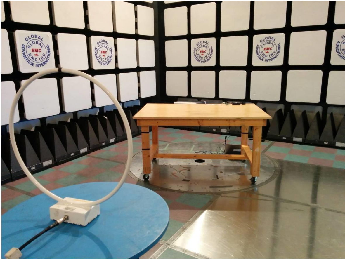
Figure 4: Radiated emission setup – photo 4
