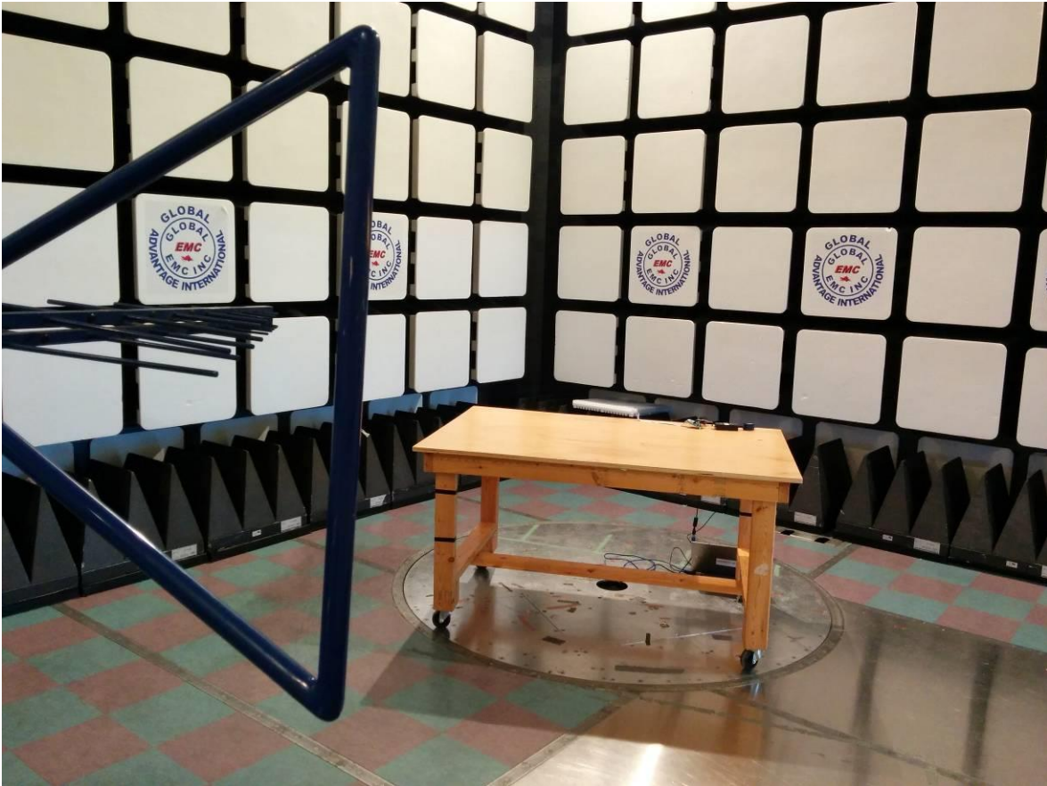
Figure 3: Radiated emission setup – photo 3
