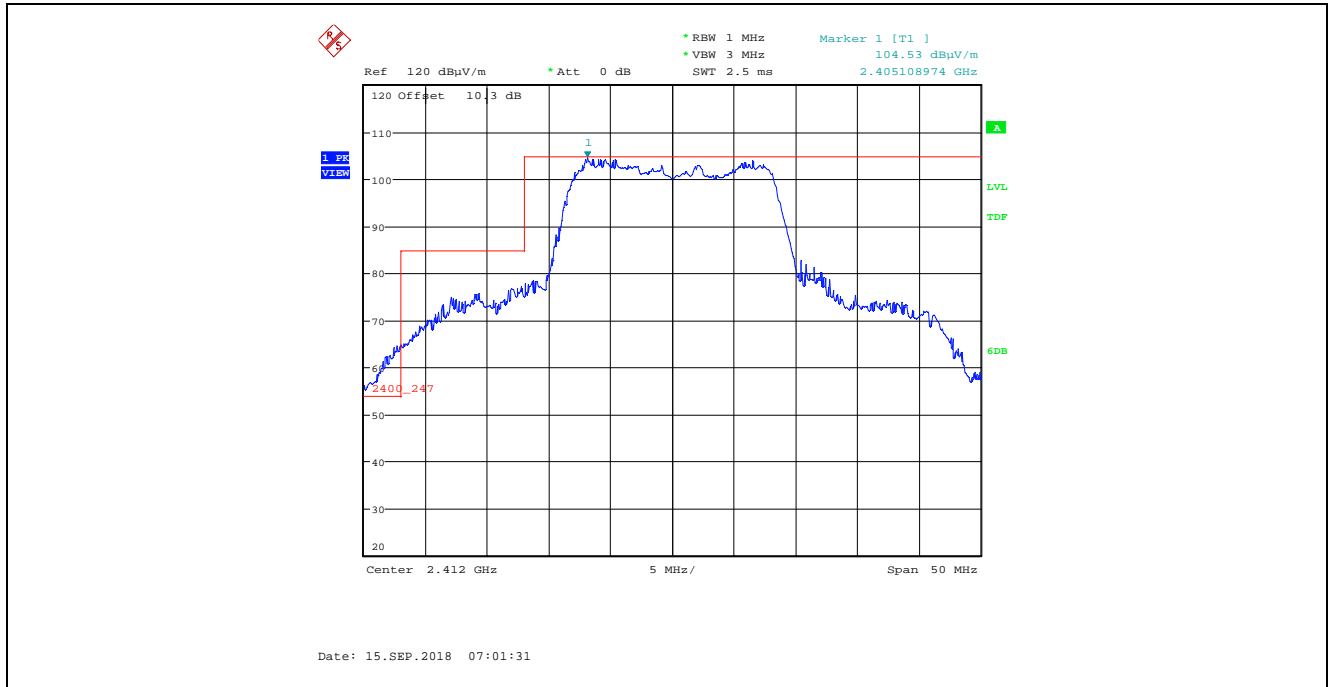
Plot 5.4.4.1.4.39. Band-Edge RF Radiated Emissions at 3 m, Vertical Polarization, Peak 18 Mbps QPSK, Power Setting 21, Channel 1, 2412 MHz
