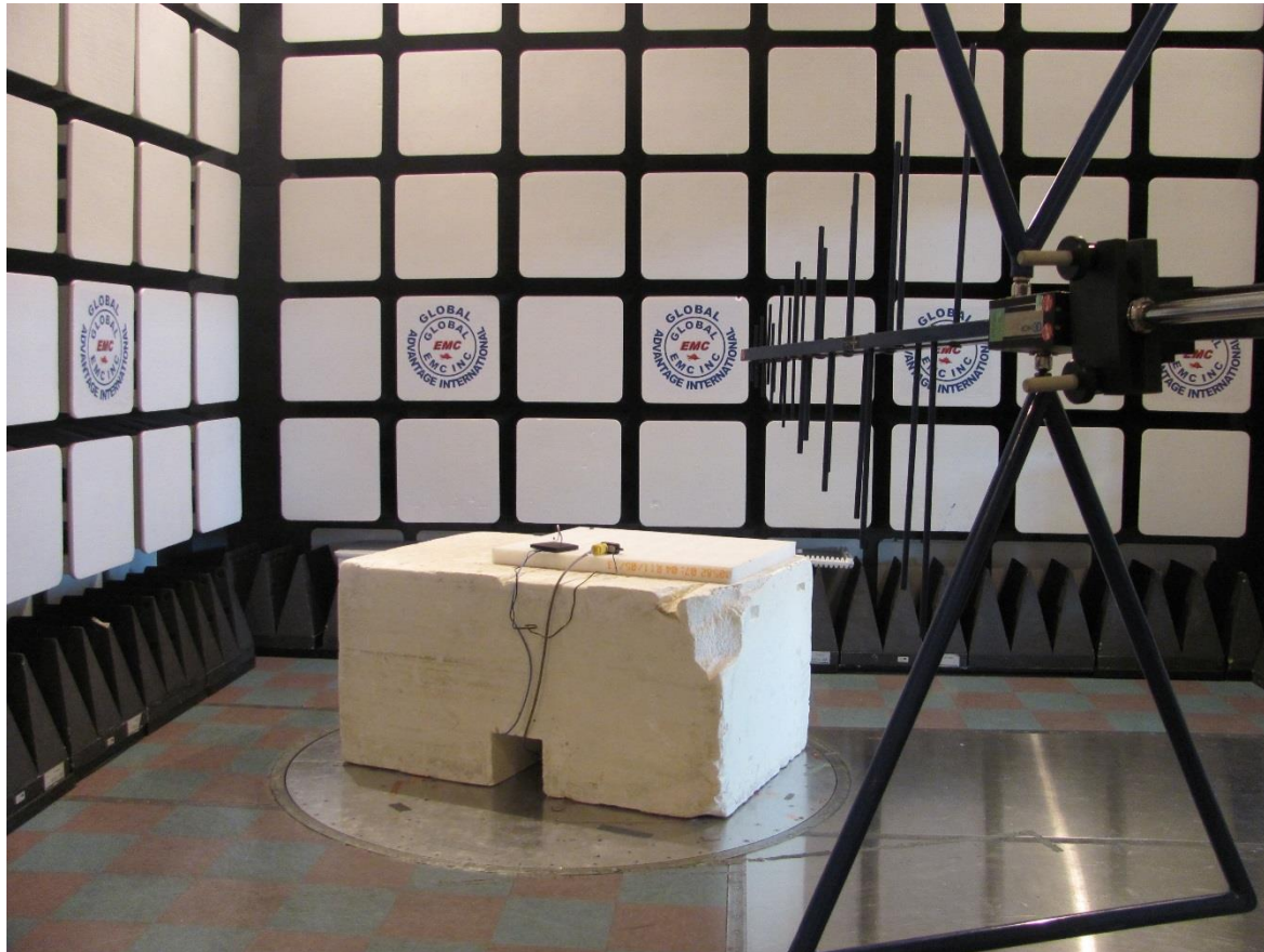
Figure 2: Radiated emission setup – photo 2
