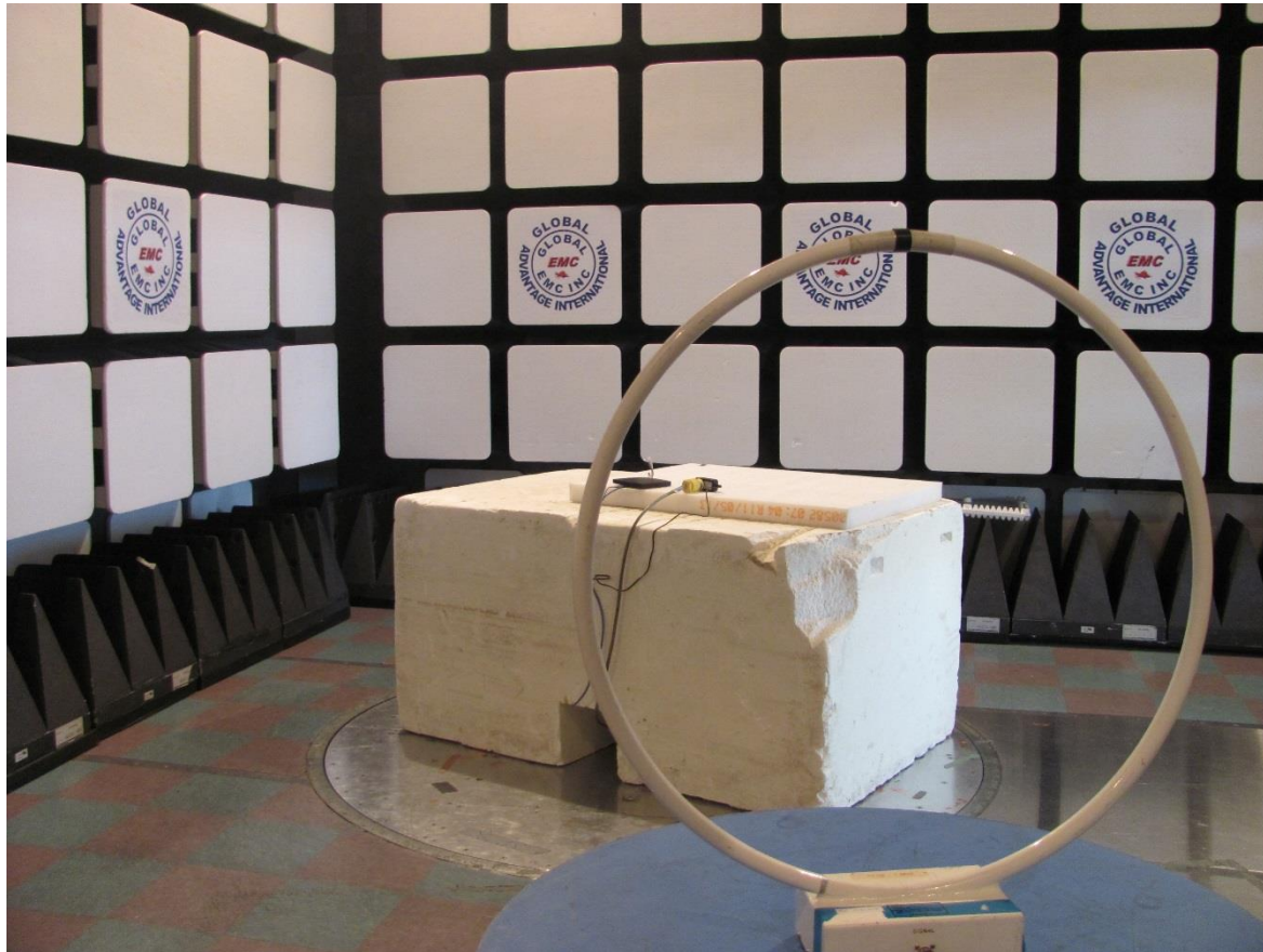
Figure 1: Radiated emissions setup – photo 1
