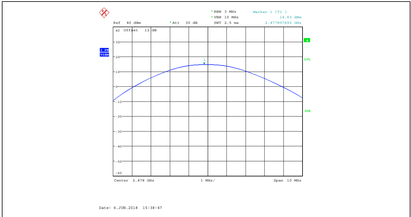
Plot 5.3.4.3. Maximum Peak Conducted Output Power, GFSK Modulation, 1 Mbps, Power Setting 200, Ch 36, 2478 MHz
