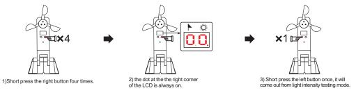
Note: In light intensity testing mode, the numerical value displays the light intensity from 1000 to 100000lx. It shows "00." below 1000lx, and "99" above 100000lx. For example, the figure "12." represents 12000lx. It will return to initial interface 3 minutes later if there is no further operation is done to the sensor.
