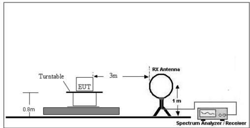
(B) Radiated Emission Test-Up Frequency 30MHz~1GHz
