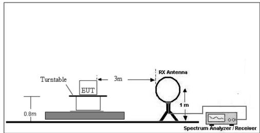
(B) Radiated Emission Test-Up Frequency 30MHz~1GHz
