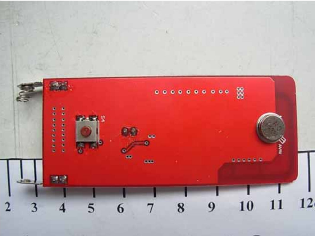
FIGURE 3 EMITTER (M/N: WSRE SERIES) MAIN BOARD (SOLDERED SIDE)
