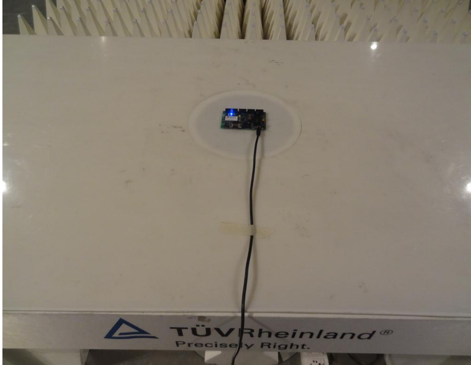
Test Setup – Module on the table(Chip Antenna)
