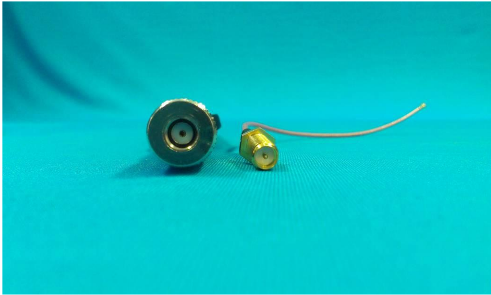
External Antenna and Cable Showing RP Connector
