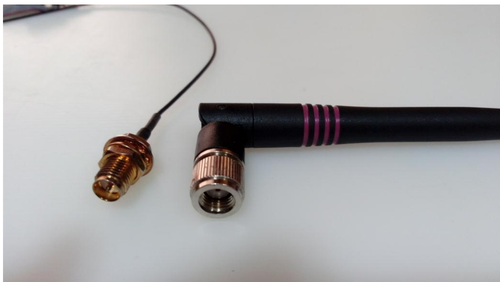
Whip Antenna – Showing RP SMA connector
