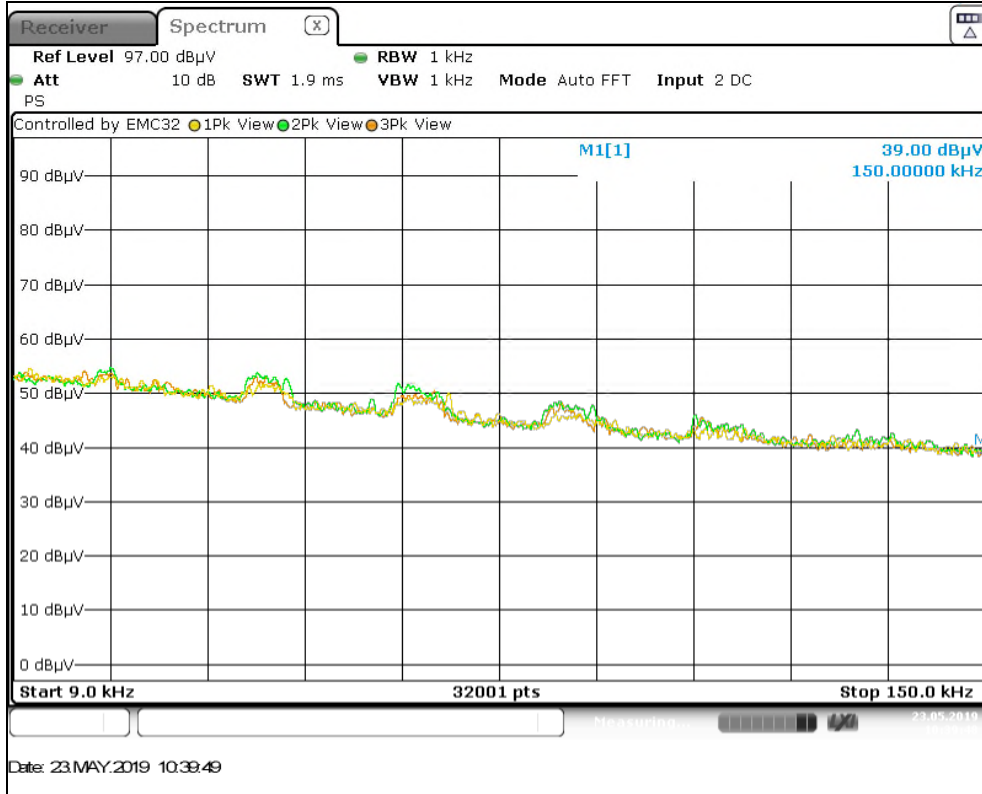
Figure A-3: Radiated Emissions – 9kHz-150kHz
