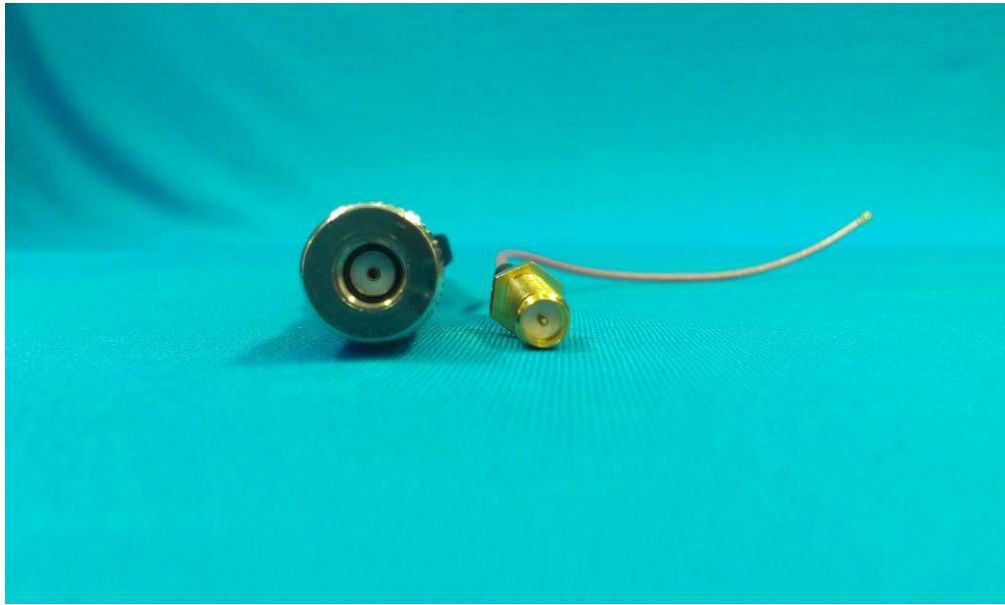
External Antenna and Cable Showing RP Connector
