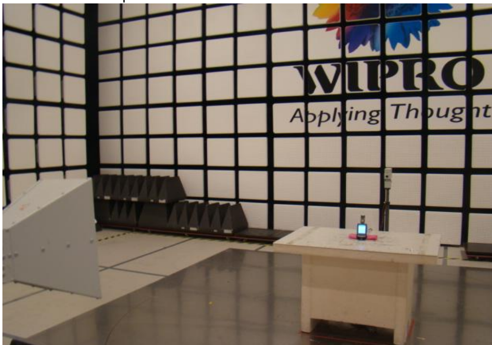
Radiated Test setup
