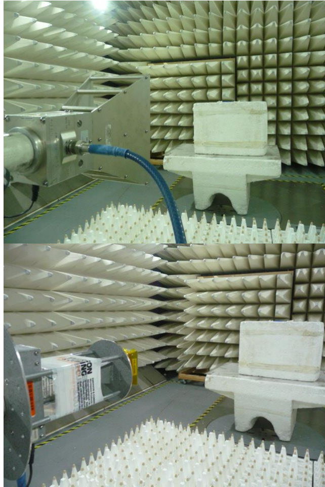
Photograph No.3, 4 Spurious and band edge emissions measurement setup in the anechoic chamber above 1 GHz
