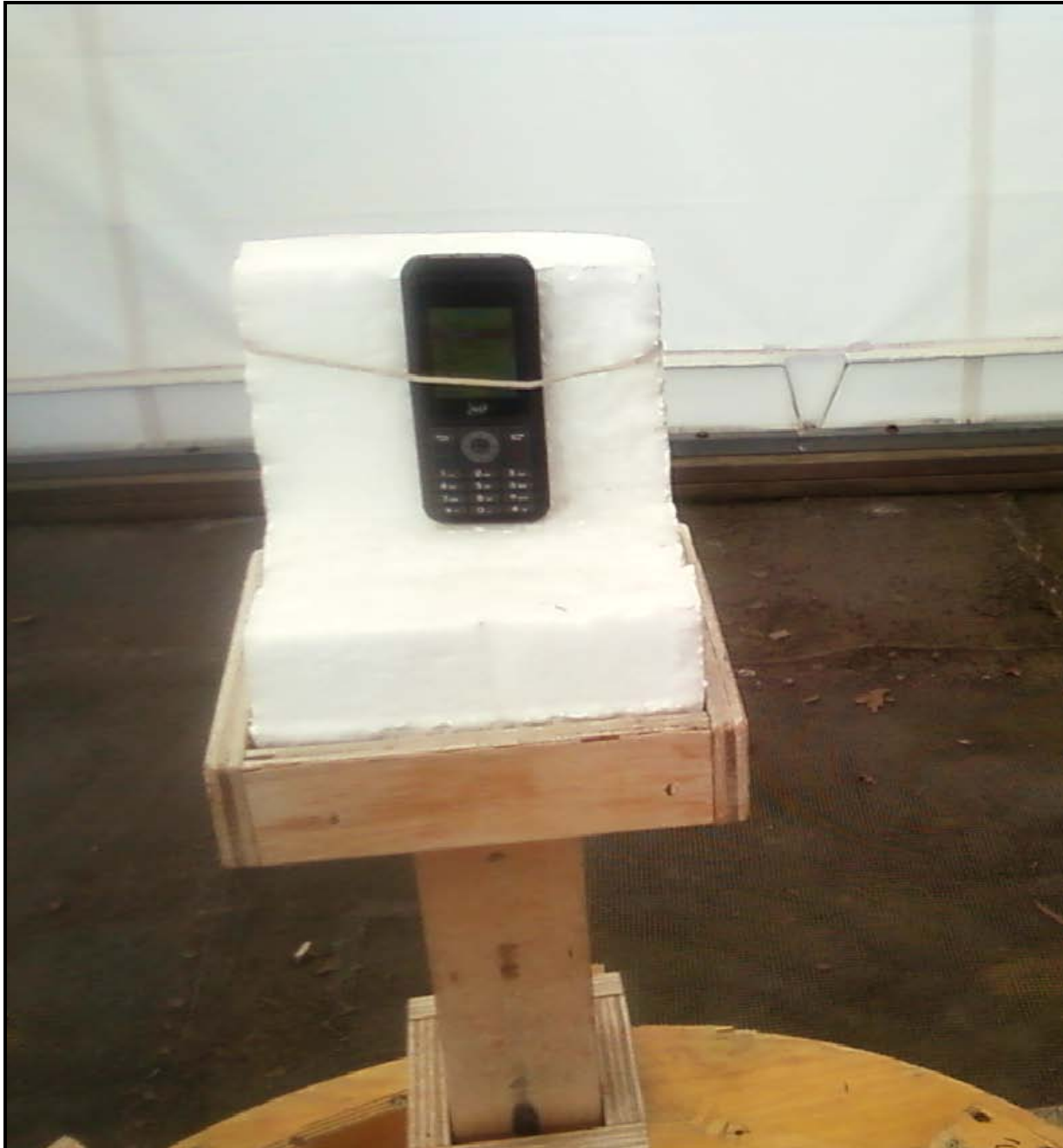
Photograph 3: Radiated Emissions – Front View
