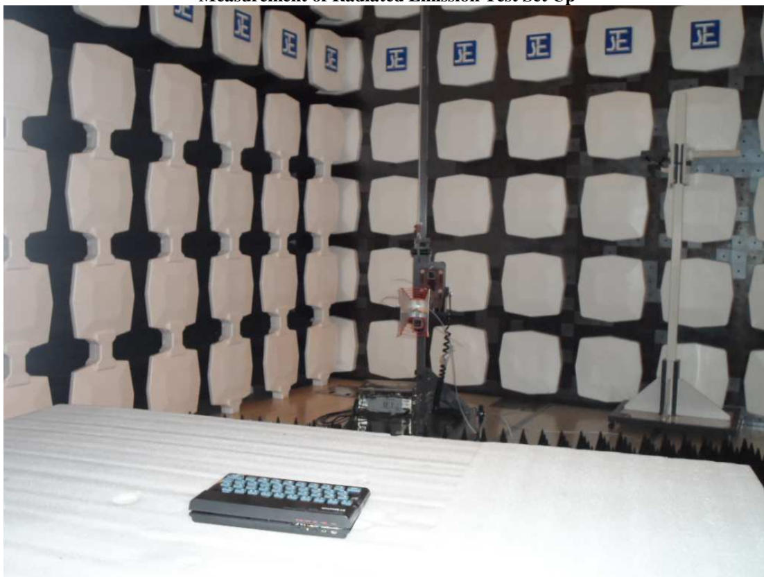
Measurement of Radiated Emission Test Set Up
