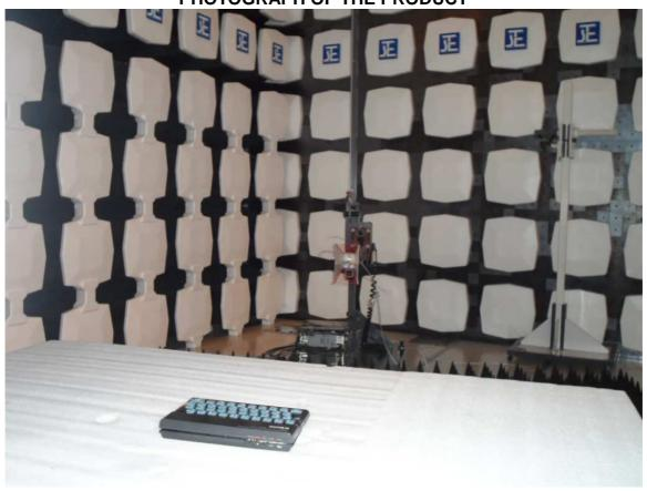
**MEASUREMENT OF CONDUCTED EMISSION TEST SET UP**
