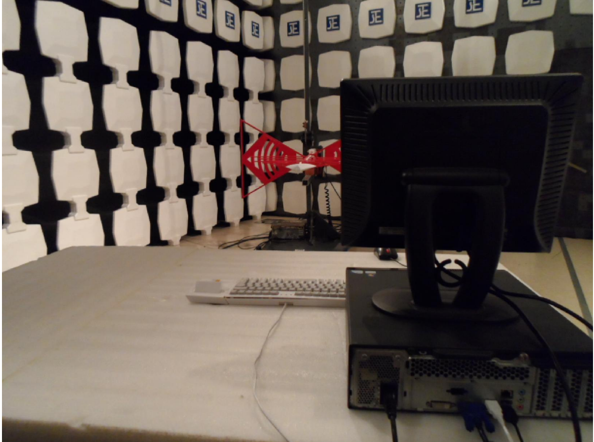
Measurement of Radiated Emission Test Set Up (30MHz – 1GHz)
