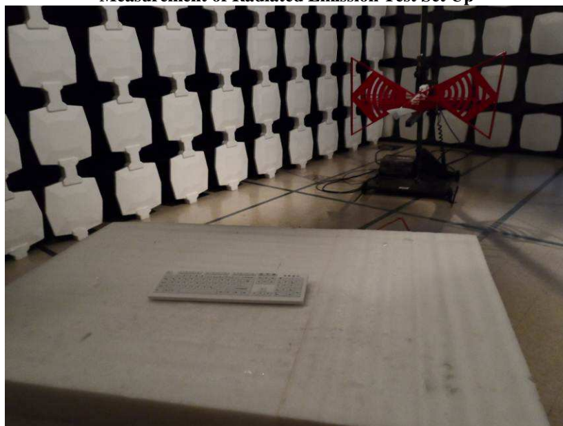
Measurement of Radiated Emission Test Set Up
