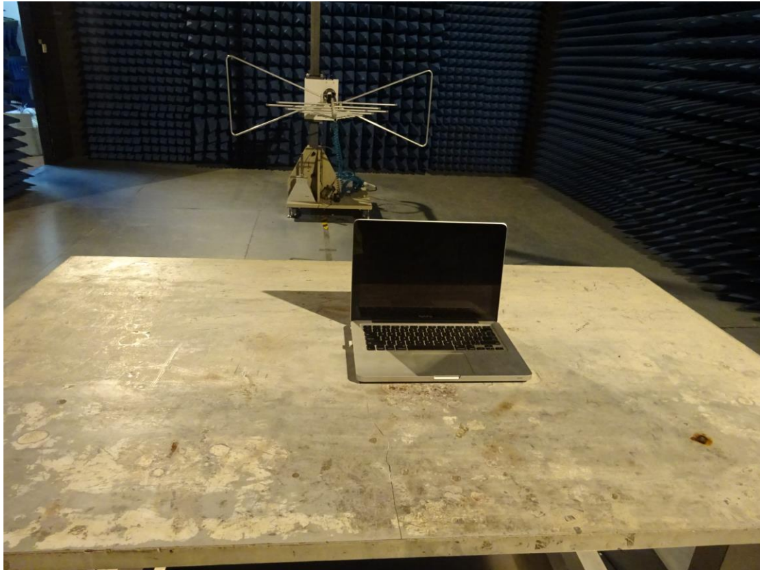
Setup photo for Radiated (below 1GHz):
