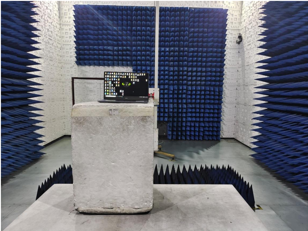
RADIATED EMISSION TEST SETUP ABOVE 1GHZ
