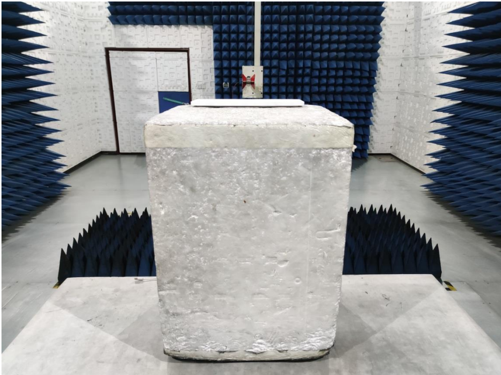
RADIATED EMISSION TEST SETUP ABOVE 1GHZ
