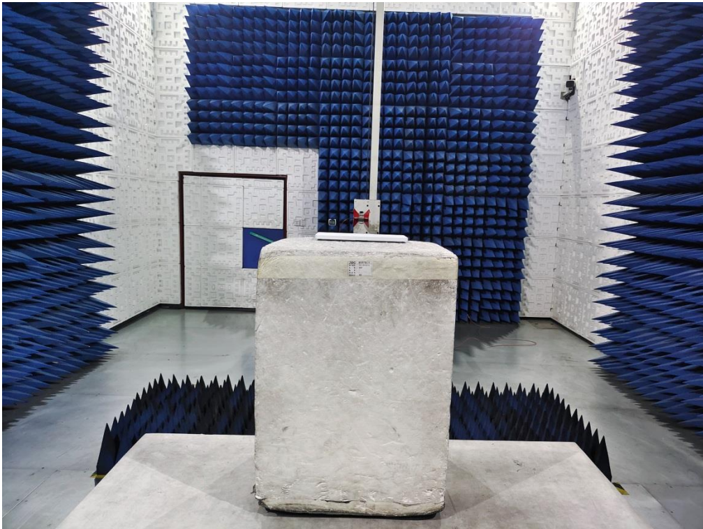
RADIATED EMISSION TEST SETUP ABOVE 1GHZ
