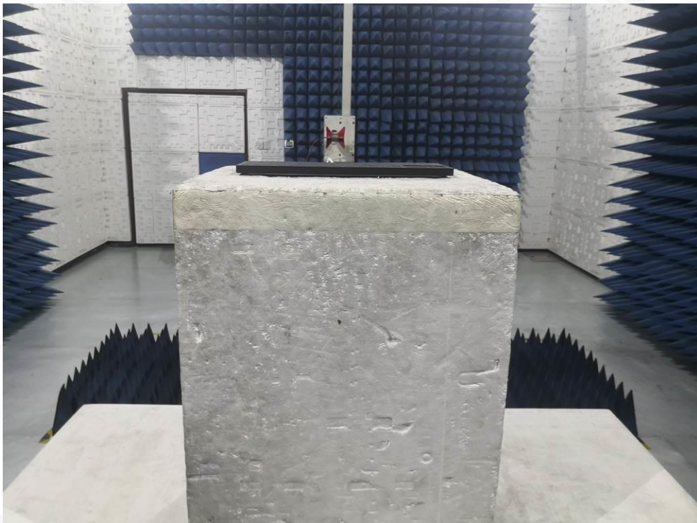
FCC RADIATED EMISSION TEST SETUP ABOVE 1
