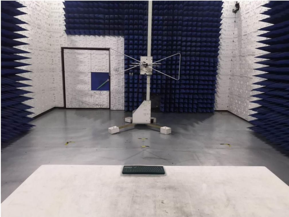
FCC RADIATED EMISSION TEST SETUP ABOVE 1
