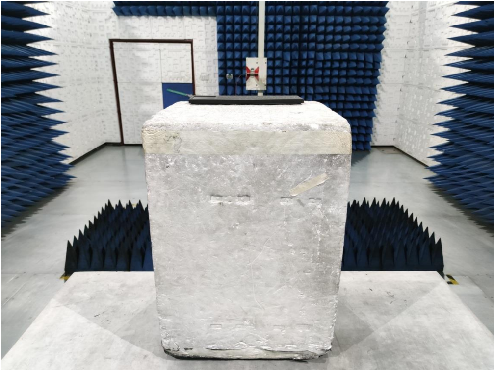
RADIATED EMISSION TEST SETUP ABOVE 1GHZ
