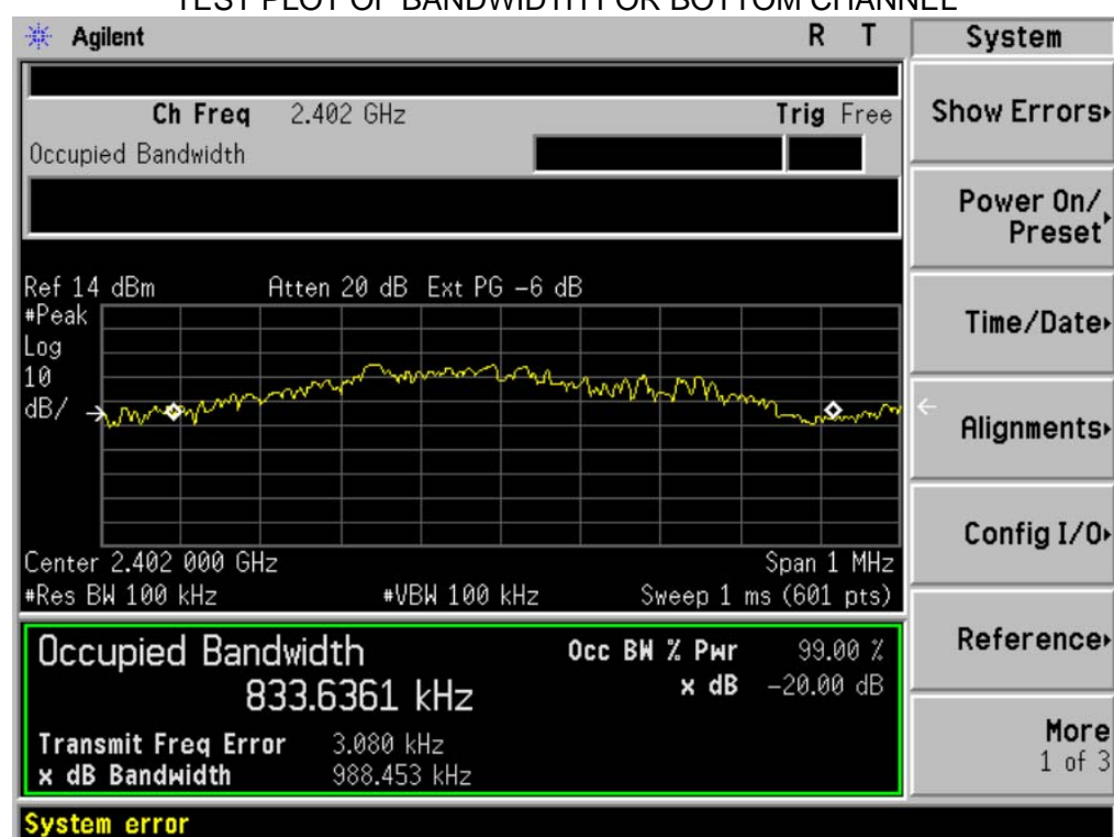
TEST PLOT OF BANDWIDTH FOR BOTTOM CHANNEL
