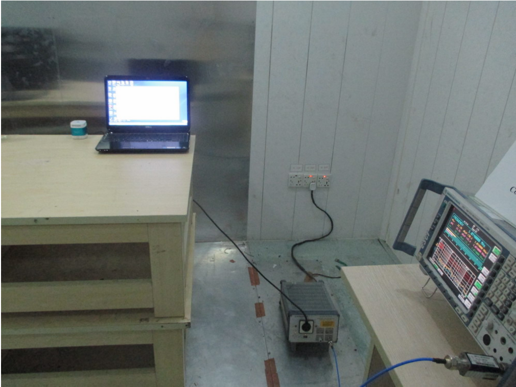
FCC RADIATED EMISSION TEST SETUP
