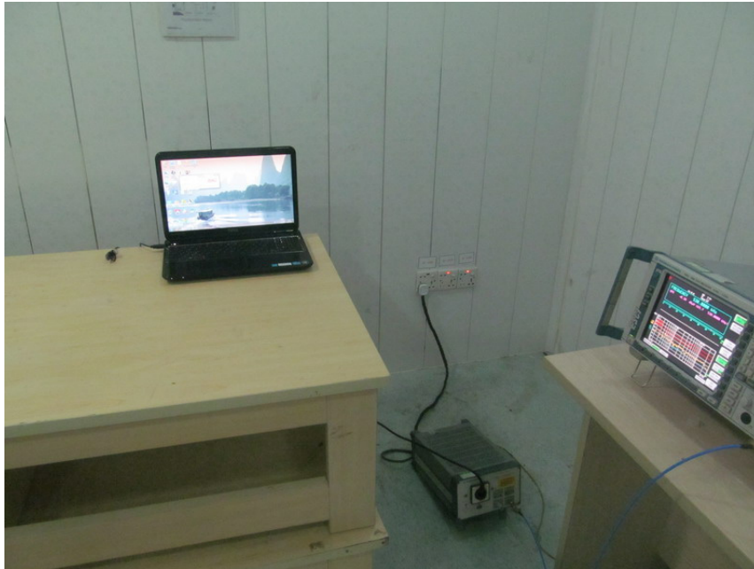
FCC RADIATED EMISSION TEST SETUP
