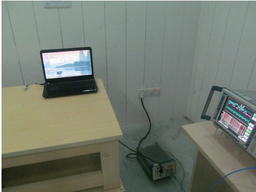
FCC RADIATED EMISSION TEST SETUP
